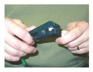
Introduce the cable into the jaws of the CS00 tool and pay attention that the cable does not lean over the stripper side
