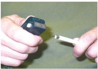
the cable correctly unsheathed looks like in the side picture where both the inner conductor and the braid are bare cleaned off Insert the plastic cap on the cable and draw back the braid over the sheath, see the attached drawing. Please note that the foil must adhere to the dielectric.
