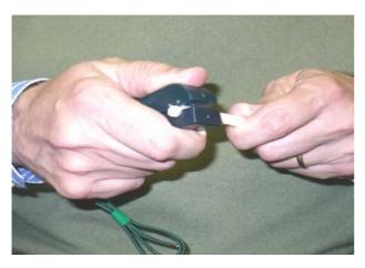
Then press the jaws heads and remove back out the cable now cleaned out by the dielectric and the outer sheath
