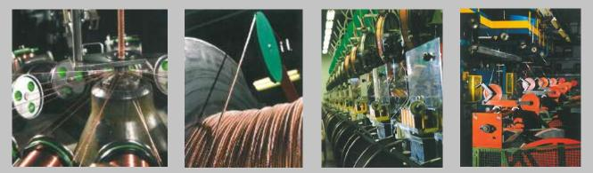
**Description:** cable shielding is formed on the primary insulation. It consists of a braid created using conductive wires, with or without interposed conductive ribbons. The company uses over 200 braiding machines, which offer great flexibility and a high production capacity.
