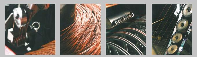
Description: red copper wires with a diameter between 0.31 mm and 3.40 mm are drawn.
